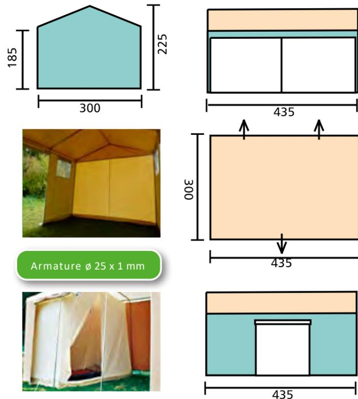
Armature  $\varnothing$  25 x 1 mm
